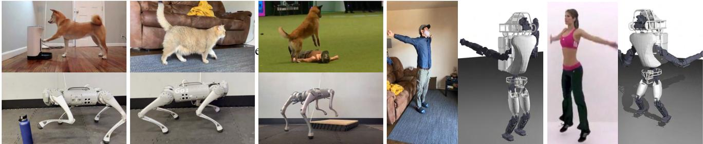
Fig. 1: A collection of video-to-robot motion-transfer demonstrations on the Unitree Go1 quadrupedal robot on hardware (left three) and the Atlas humanoid robot in simulation (right two). From left to right: a dog reaching for a water feeder with one of its front feet, a house cat pacing, a trained dog performing a Cardiopulmonary Resuscitation (CPR) exercise on its human partner, a human stretching his body and limbs, and a human demonstrating a jumping-jack exercise.
