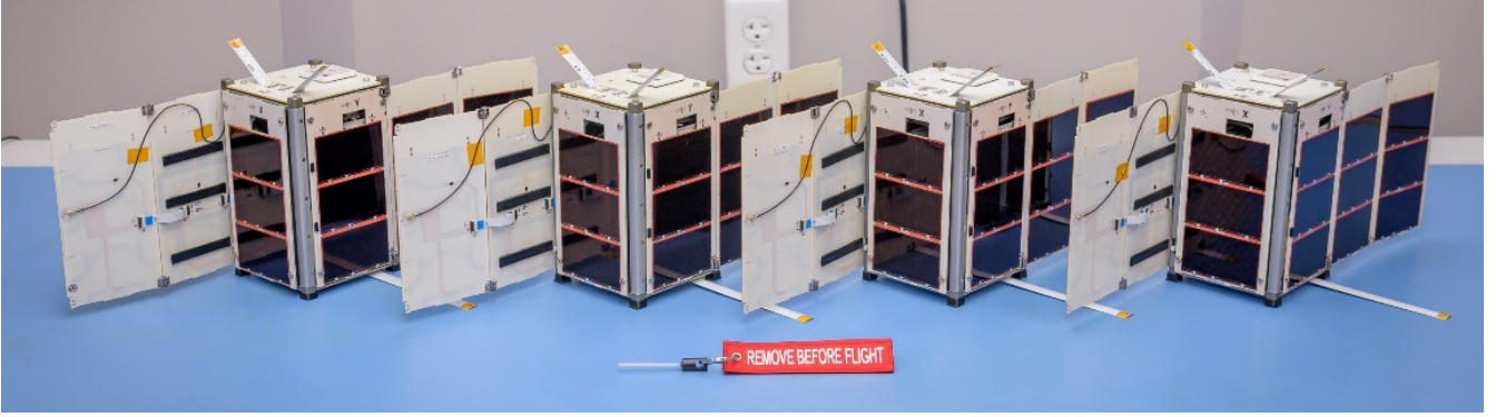
Figure 2. The four PY4 satellites, a collaboration between Carnegie Mellon University and NASA Ames Research Center, were launched on March 4, 2024 on the SpaceX Transporter 10 mission and deployed on a sun-synchronous orbit. The 1.5U satellites demonstrated a suite of novel navigation and control algorithms for low-cost platforms [14].
