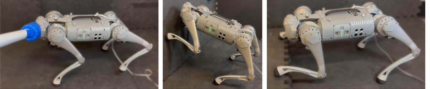
Fig. 1: Hardware demonstrations on a Unitree Go1 quadruped: stable trotting while being pushed (left), transitioning from ground to standing against a wall (center), and placing two feet onto a step (right).
