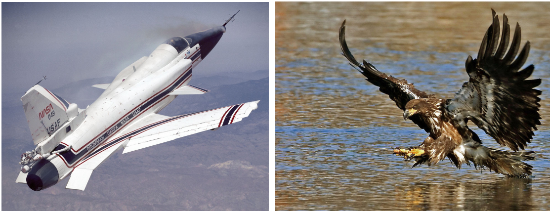
Figure 1. Forward-swept wings in aviation and in nature. Left: The Grumman X-29 experimental aircraft flying at a high angle of attack. Right: A brown eagle sweeps its wings forward during a “snatching” maneuver.
