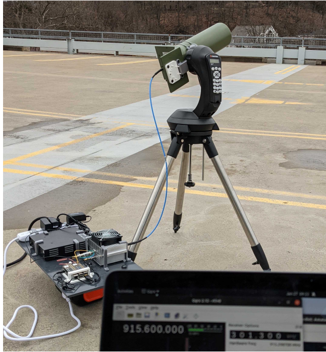
Figure 10. V-R3x mobile ground station. A low-cost amateur telescope go-to mount is used automatically point a 12 dBi gain 915 MHz helical antenna using standard open-source satellite-tracking software. The antenna is connected to a pair of LoRa radios through a low-noise amplifier for receiving and a 50 W power amplifier for transmitting. The entire setup is portable, can be assembled and disassembled in minutes, and can be powered from a lithium-ion battery pack.
