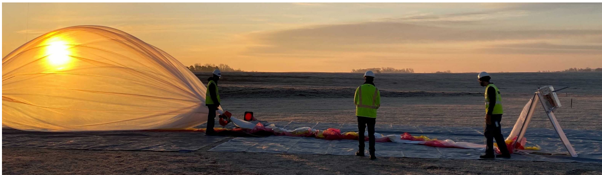
Figure 8. Launch of the V-R3x high-altitude balloon test on March 12, 2021. A single V-R3x CubeSat is mounted inside the balloon payload seen on the stand in the right of the photograph.
